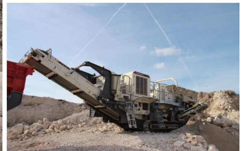
NFJ1060硬岩骨料头破处理应用 NFJ1060 crushing hard rock in primary stage
