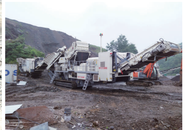
NFC1300E应用于玄武岩破碎 NFC1300E hard rock application
